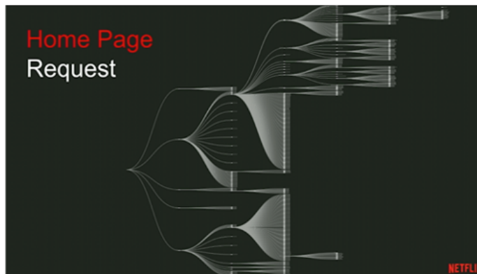
Figure A.1 Illustration of request fan-out to downstream services that occurs on a request to get Netflix's homepage. Image from https://www.oreilly.com/content/application-caching-at-netflix-the-hidden-microservice/ .
